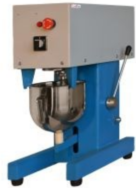
Cement Mortar Mixers
